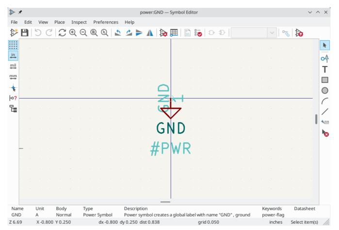
Power port symbols consist of a pin of type "Power input" that is marked invisible. They must also have the "Define as power symbol" property checked. Invisible power input pins have a special property of making implicit global connections based on the pin name.
